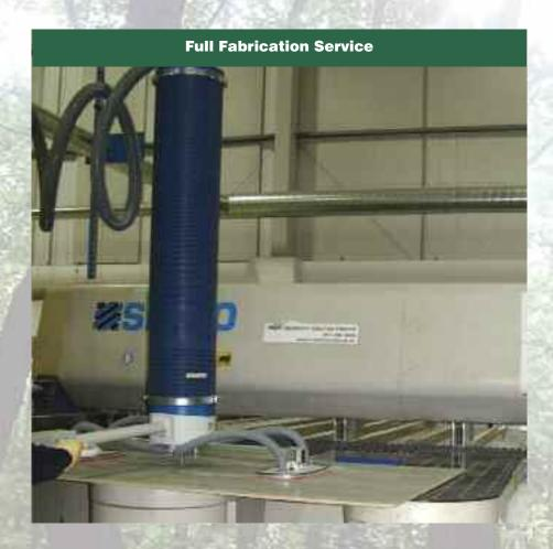
Versapanel is a class '0' cement bonded particle board comprising of wood particles and cement.
