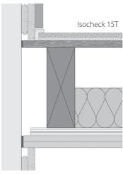
Flanking Strip turned back under skirting and trimmed flush with a sharp knife.
