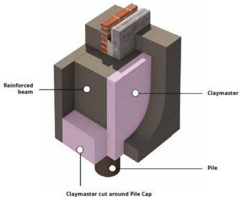
Claymaster is an EPS compressible-fill material which can be used to prevent potential problems in foundations due to moisture movement in soils which contain a large proportion of mineral particles below 0.002mm ('clay heave'). The material can be used as permanent shuttering for cast in-situ reinforced concrete, reducing pressure on ground beams in piled foundations, and on the sides of trench fills.
