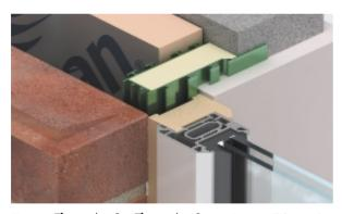
Kingspan Thermabate® or Thermabate® PLUS "reversed" for use in flush or check reveal details
