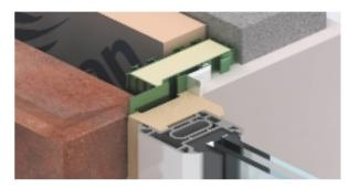
Kingspan Thermabate® or Thermabate® PLUS in position with reveal clip engaged behind window frame.
