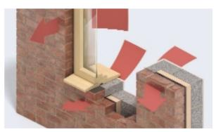
Heat loss paths around a typical window opening – traditional construction
