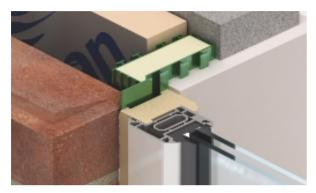
Kingspan Thermabate® or Thermabate® PLUS with fixing flange set on outer leaf
