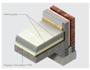
Figure 10 - 24 Hour heating applications - below the floor slab
