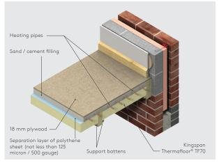
Figure 14 - Intermittent heating applications - suspended timber floor
