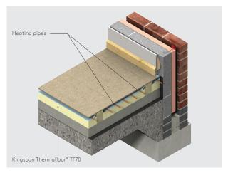
Figure 12 - Intermittent heating applications - timber floor on battens
