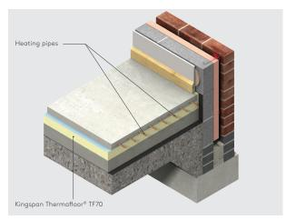
Figure 11 - Intermittent heating applications - below the floor screed
