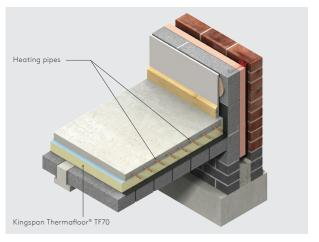
Figure 13 - Intermittent heating applications - beam and block floor
