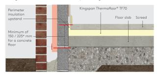
Figure 1 - Complete masonry floor insulation
