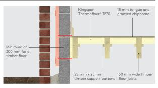
Figure 9 - Complete timber floor insulation
