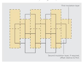
Figure 15 - Offsetting of multiple insulation yayers
