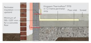
Figure 2 - Perimeter strip masonry floor insulation
