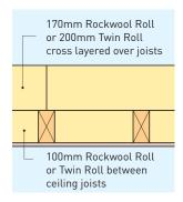
Figure 1 Cross layered RollU-value 0.16 W/m<sup>2</sup>K
