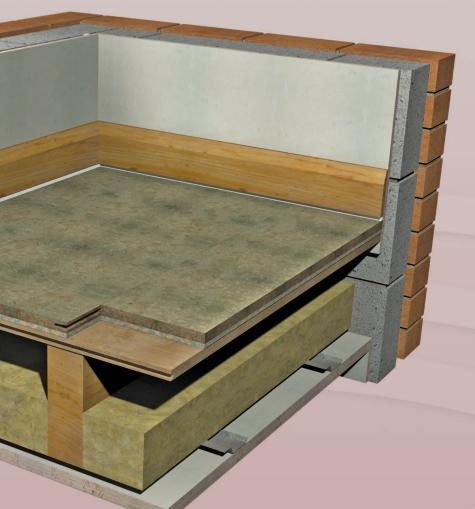
OVERLAY PLATFORM SYSTEMS DIRECT TO FLOORBOARDS
