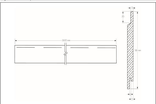
1.3 The planks are fixed back to the substrate by means of stainless steel Cedral Click Clips (see Figure 2) which are attached back to vertical timber battens or metal profiles by means of stainless steel screws (timber) or rivets (metal).
