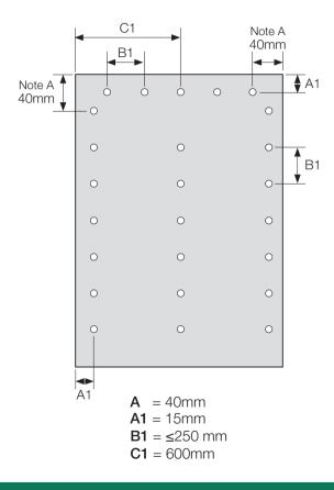
Install with stainless steel countersunk head screws adapted to substrate. Minimum - length 36mm and diameter 3.5mm.
