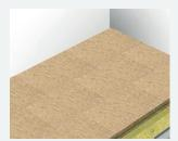
All joints to be glued, on all sides of the panel to give the best bond. Adhesive not to be spared.
