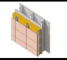
In line with the Building Control Alliance Technical note 18; 'use of Combustible Cladding Materials on residential buildings paragraph 12.7 of AD B2' - use materials of limited combustibility throughout the cladding system.
