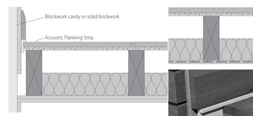
Flanking Strip turned back under skirting and trimmed flush with a sharp knife.
