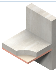
Insulation for structural ceilings (soffits)
