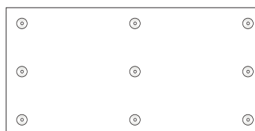
9 No. per board (2.4 x 1.2 m board – 3.12 fixings / m 2 )
