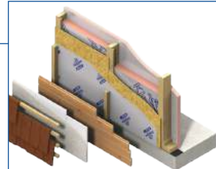
Insulation for timber and steel framing systems
