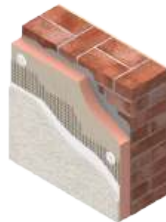
External insulation for masonry walls
