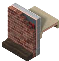
Full and partial fill cavity wall insulation
