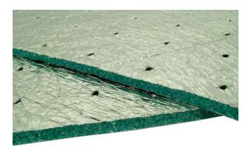
Low-E® PERF is the ORIGINAL breathable reflective foil insulation. With a Moisture Vapour Transmission Rate (MVTR) of less than 0.25 MN s/g, Low-E PERF is Certified for use in roofs, walls and floors where breathability is required.Low-E® PERF is recommended for use on the external sides of a building envelope or in a loft space over existing insulation.
