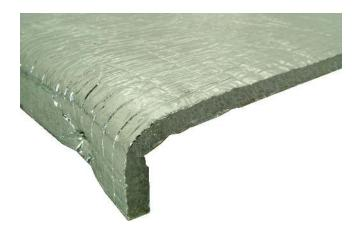
Low- $E^{\otimes}$  TAB is our standard Low-E material, pre cut for your convenience to fit neatly between rafters, joists and studs. Low- $E^{\otimes}$  TAB is manufactured in 400mm and 600mm wide rolls. (3x 400mm Rolls per pack) or (2x 600mm Rolls per pack). Low- $E^{\otimes}$  TAB should be put in place and then stapled through the TAB to hold it in place.
