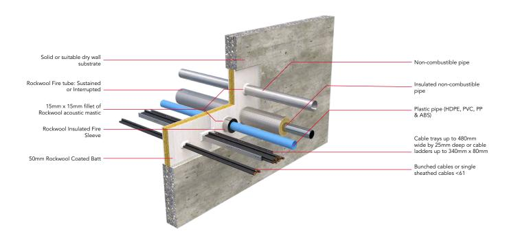
For a comprehensive range of ROCKWOOL solutions for penetrating services passing through the Ablative Coated Batt, please refer to the applicable ROCKWOOL standard details available at www.rockwool.com/uk or contact ROCKWOOL Technical Solutions.
