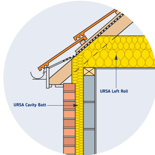
**Figure 8 – Cold Pitched Roof – Gable Detail**
