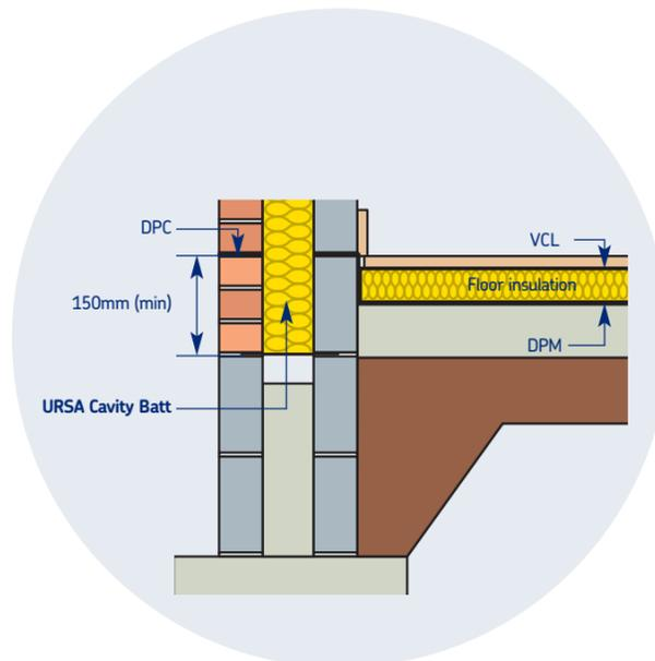
Figure 1 – Wall/Floor Junction – Insulation Below Slab
