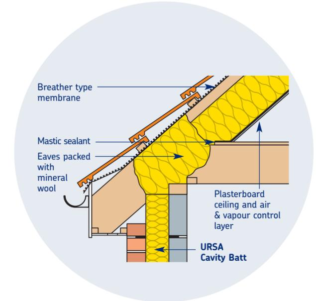
**Figure 10 – Warm Pitched Roof – Gable/Verge Detail**
