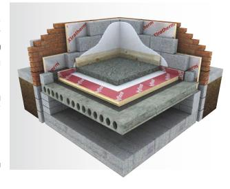
Detailing at wall/floor junctions is essential to reduce thermal bridging. By placing an upstand of Xtratherm Perimeter insulation 25mm thick around the external and internal wall/floor junctions, a robust detail is created.
