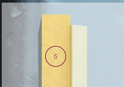
5. High performance core - 0.021 W/mk Thermal Conductivity.
