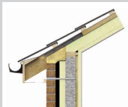
Improvements in U-values and accredited detailing can be achieved with an additional layer of an Xtratherm Thermal Liner. (See table for U-values)
