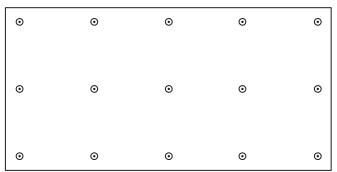
15 fixings per board (5.20 fixings / m2)
