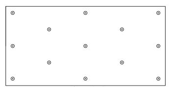
13 fixings per board (4.51 fixings / m2)
