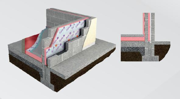
SR/CW partial fill cavity wall insulation is the solution of choice to achieve the lower U-Values asked for under the building regulations whilst maintaining a residual cavity as a protection from wind driven rain.
