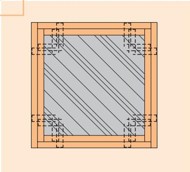
2 layer timber support lining F 60-B for 4-sided exposure to fire
