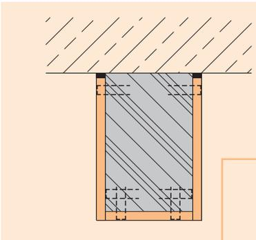
3 layer steel beam encasement for 4-sided exposure to fire
