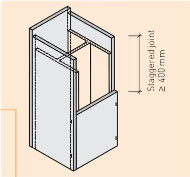
Encasement of a steel support for 4-sided exposure to fire
