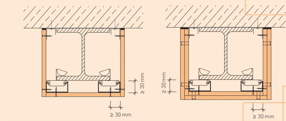
Single-layer steel beam encasement for 3-sided exposure to fire
